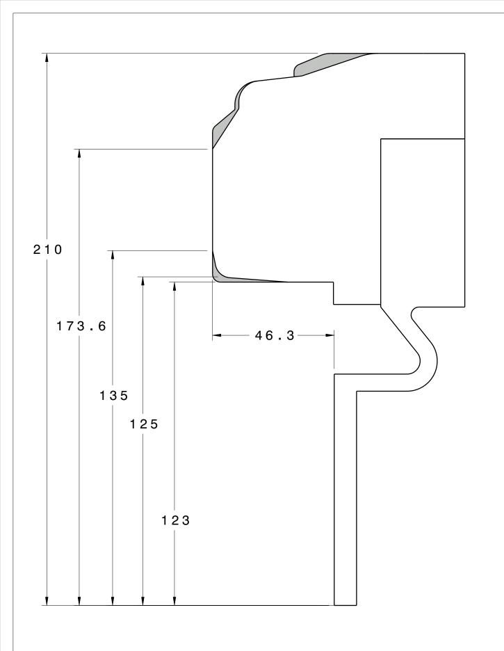
SHADED AREAS INDICATE ADDITIONAL CLEARANCE NEEDED FOR SYSTEMS USING GTR CALIPERS ("R" SUFFIX SYSTEMS)
