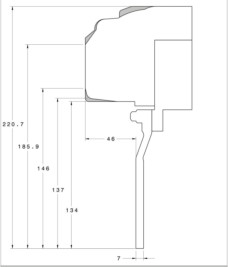
SHADED AREAS INDICATE ADDITIONAL CLEARANCE NEEDED FOR SYSTEMS USING GTR CALIPERS ("R" SUFFIX SYSTEMS)
